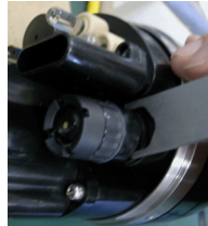
Undo a DO sensor from the sensor probe
